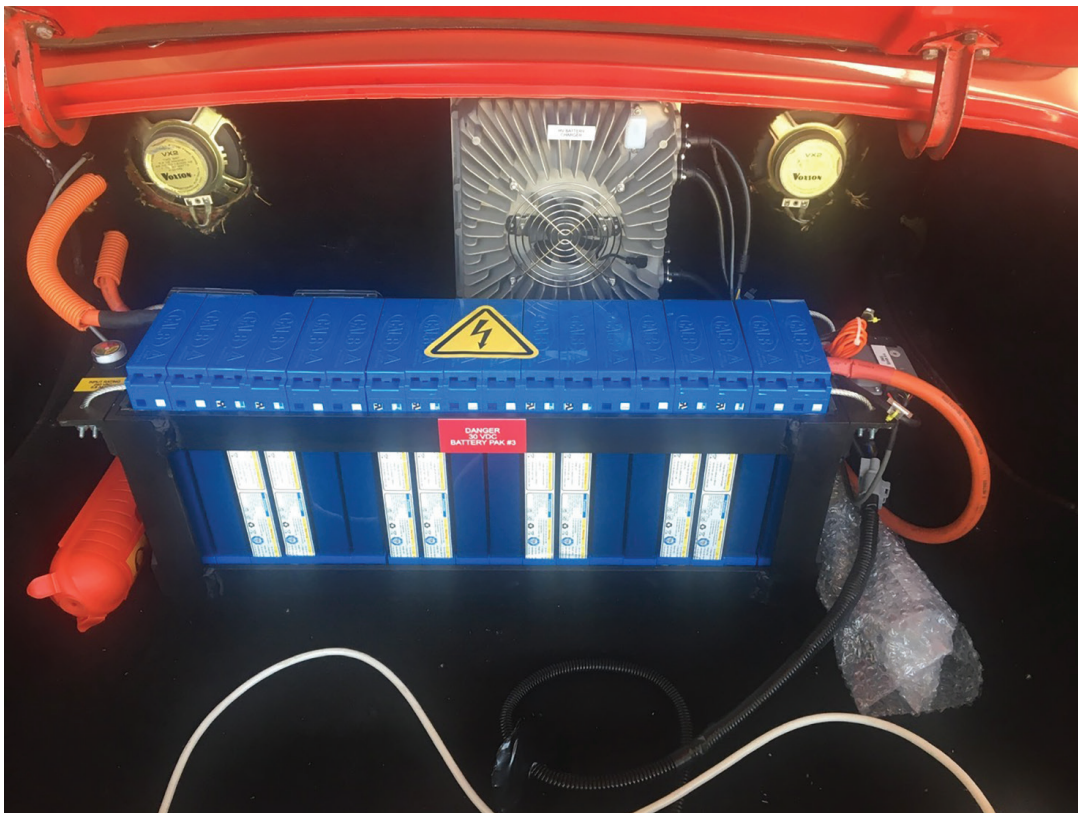
Batteries in boot, showing plastic protection headers and battery charger
